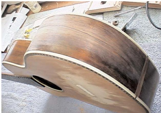
Now that all the interior work was done and the cracks repaired and/or stabilized, it was time to begin preparing the surface for finishing. This is best done before the bridge is attached so it is easier to go over the whole surface.
