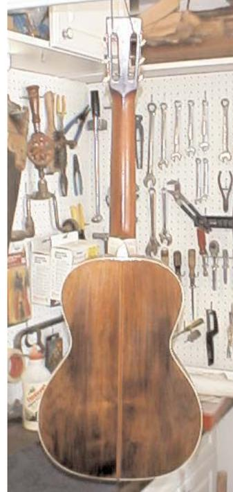
On Day 9, I started the finish process. I used a slightly colored tung oil on the top and uncolored tung oil on the sides and back. To protect the fingerboard and neck where it attaches to the body, so as not to get any additional varnish on it, I taped the area with a painter's masking tape.
