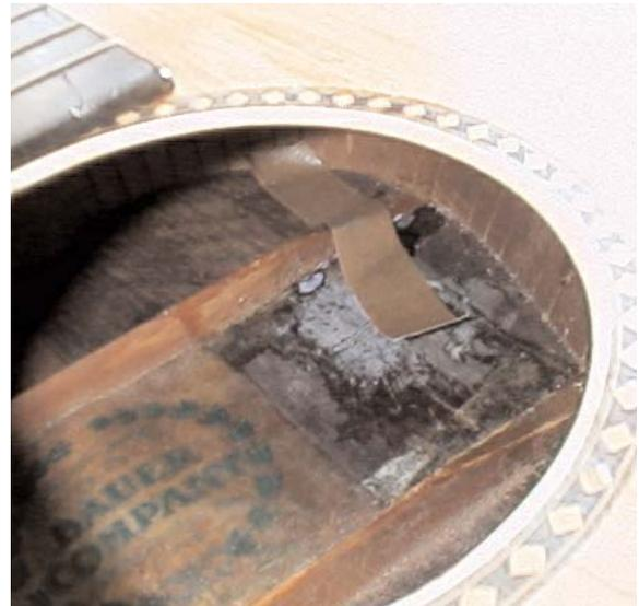
On day 4, I worked on stabilizing the largest back crack and the back braces. I applied several wood cleats over the crack so it couldn't get any worse. The wood has shrunk too much over time to be able to close it up fully, but the cleats will protect it.
