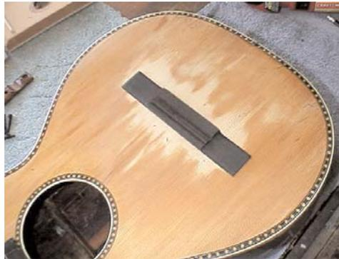
On Day 3, I started on the bridge work. These pictures show the 1/8" thick maple piece I cut to strengthen the bridge plate, the peg holes that I'll patch later, and a new carved ebony classical style bridge.
