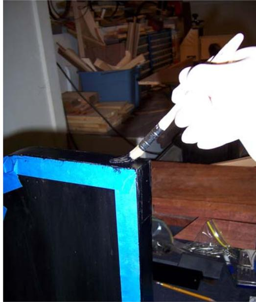
With the back finished, I needed to touch up the sides where I had closed up the failed glue joints. The sides originally had a glossy finish, just like the tail pin cover, so I used the same glossy black enamel to recoat and touch up the sides. This was another three coat, three day project.
