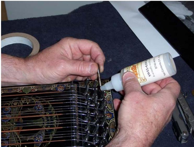
Often when removing zither tuning pins, the holes seem to expand. When reinstalling the pins, several often don't have the friction to hold a tightened string. There is an interesting liquid product called Swellock, that can actually swell the wood to make parts fit tighter. It's usually used on chair tenons to tighten loose joints, but I've been able to use it on tuning pin holes to make the pins fit tighter.
