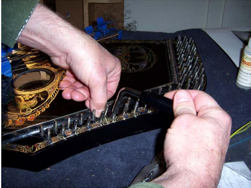
The next day, I began re-stringing the zither. With the number of strings, and the effort it took to restring, I spaced it out over two days. I had taken photos of the zither before I started removing the strings so I would be sure to place the double strings properly over the single guide pins. The double string setup on this Slovenian instrument is very different than others I've seen.
