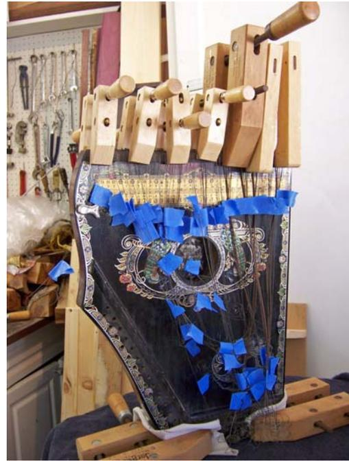
There were only a couple of places where the glue joints had failed, and this was probably due to having it stored over the years with the strings tightened. This caused the zither to rack slightly and pulling part of the cover away from the tuning pin block area. The failure was not that bad and the separation was not very large.
