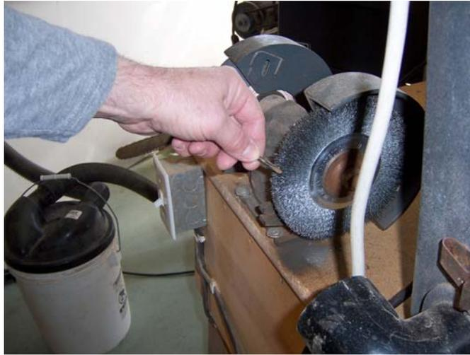
Day 3 was spent buffing and polishing the tuning pins. I used a wire wheel to buff off the corrosion. This took a few hours to do since there are 62 tuning pins on this particular zither. Most zithers have single melody strings and usually have a total of approximately 36 to 48 strings. This Marat, on the other hand, has double courses of each melody note. This gives each note a much fuller sound and a little more volume.
