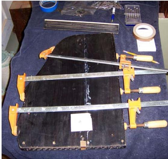
On Day 5, I worked on the back crack. Cracks are very common on these old zithers due to the constant expansion and contraction wood goes through during a year of dampness and dryness. This zither's crack, even though it ran the length of the back, was not separated very much and that made it fairly easy to inject glue into it and lightly clamp it together.
