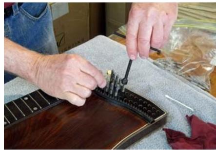
When I started to reinstall the tuning pins, I noticed that they slipped in too easily. Loose fitting pins could easily slip when the strings are installed. To fix that, I use a special liquid that swells the wood. This liquid is usually used for fixing loose chair rungs and legs, but works quite well with tuning pins.
