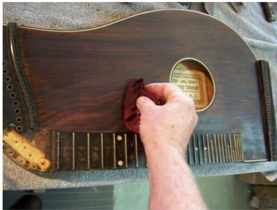
Now with the top and sides smoothed out, and the patches touched up, I spent several days applying a tung oil varnish. This type of finish can be applied only once a day. It needs to dry around 24 hours between coats. I applied four coats.
